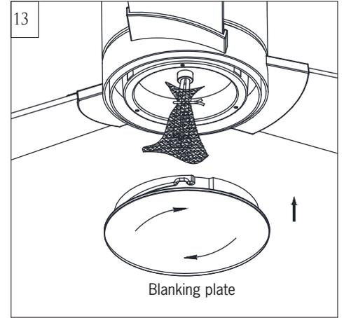
Attach a blanking plate by locating dimples in light pan with grooves on the blanking plate and twist clockwise until tight.
