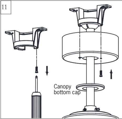
Partially loosen one and remove one preassembled screw from mounting bracket. Save screw. Lift canopy up, aligning its keyhole slot with the preassembled screw on mounting bracket and twist clockwise to lock in place. Reinstall the screw removed and tighten all screws securely. Attach canopy bottom cap onto canopy by aligning its notch with the screws on mounting bracket and twist clockwise till tight.
