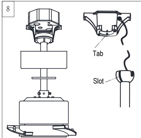
Install ball end of downrod into mounting bracket opening. Align (engage) slot on ball with tab on mounting bracket.
