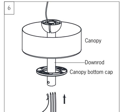
Place downrod over canopy and canopy bottom cap. Thread lead wires and safety cable from motor assembly through downrod.
