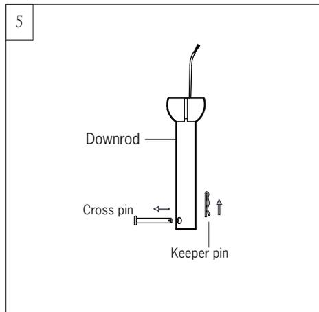
Remove preassembled cross pin and keeper pin from downrod. Keep parts.
