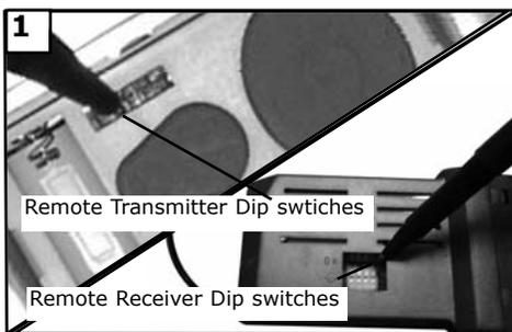
Remote Transmitter Dip switches
