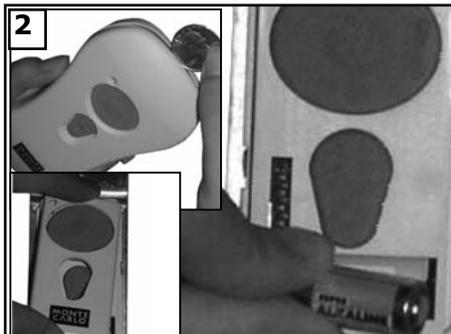
Remove cover by snapping off from top or bottom. Remove battery cover. Install 12V battery into wall remote. Duracell MN21 / Eveready A23 / GP 23A all 12V. Attach cover of remote by placing over buttons and snap the battery cover in place.
