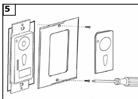
Attach front cover to wall control with screws provided. Snap battery cover in place.
