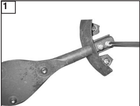
1 Attaching blade arm to fan heel.
