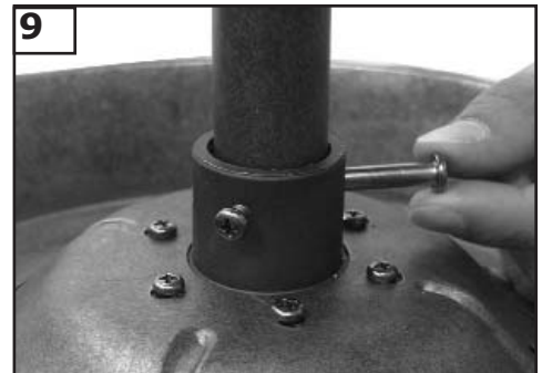
Insert downrod into yoke on top of the Fan body. Align the hole in the downrod with the hole in the yoke. Insert the pin through the yoke and downrod until the point appears on the other side.
