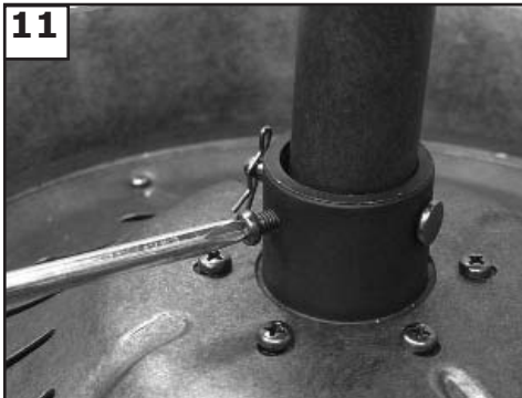
Tighten the 2 set screws on the yoke once the downrod is in place.
