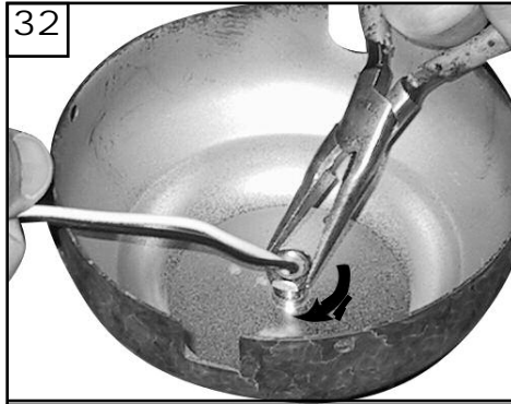
32 Install keeper nut from the threaded pipe of the light kit.
