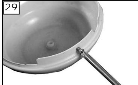
29 Remove 3 screws on the ridge of the switch cap and save.
