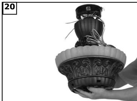
20 Hang assembled fan from the mounting bracket installed to ceiling in previous step. Make sure the fan is hanging straight. Rotate fan until the tab on the Mounting bracket engages the slot on the Downrod Ball. This must be done to prevent the fan body from rotating when the blades are in motion.
