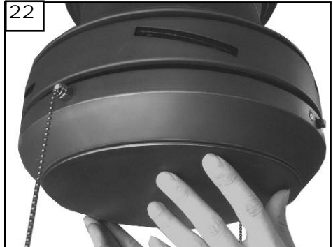
22 Attach the non light cover by locating dimples in the light fixture with the grooves in the non light kit cover and twist clockwise till tight.
