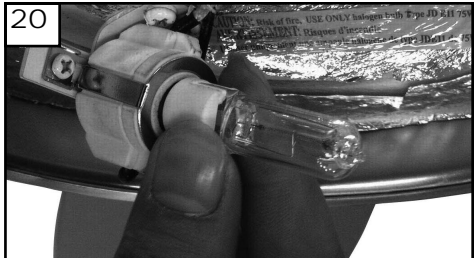
20 Install 75 watt halogen bulb. Do not touch bulb surface as oily residue from skin can cause the bulb to explode. Bulb Included. WARNING: Over lamping the fan will result in the fan lights shutting down until the proper wattage of bulbs are installed. Reset the lights by turning off the wall switch, breaker, or by remote. Replace bulbs with the correct wattage bulbs, turn the power on.
