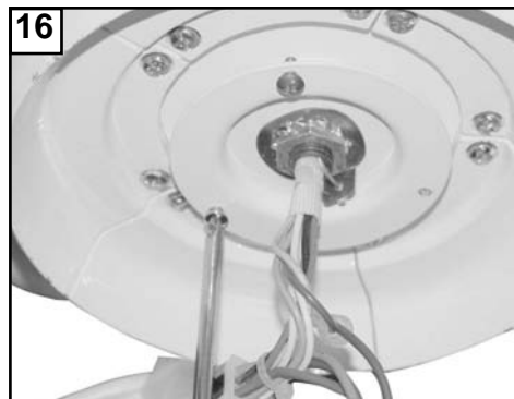
16 Loosen 2 screws with key slots and remove 1 screw without slot from motor plate and save screw.
