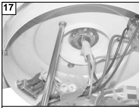
17 Install switch housing plate by twisting plate with key hole slots into place. Replace screw removed and tighten the 3 screws securely.
