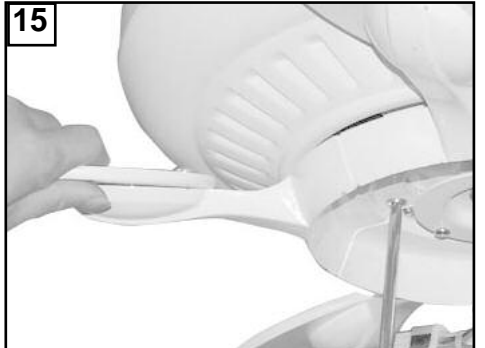
15 Check the motor for plastic shipping stabilizer tabs and remove them if they are present. The screws, washers, and motor pads are pre-installed to the blade holders. Attach blade assembly to motor and tighten screws securely.
