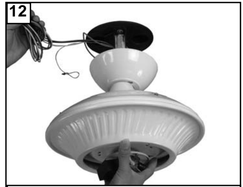
12 Carefully lift fan assembly onto mounting bracket. Rotate fan so that the notch on the ball engages the ridge in the mounting bracket. This will allow hands-free wiring.
