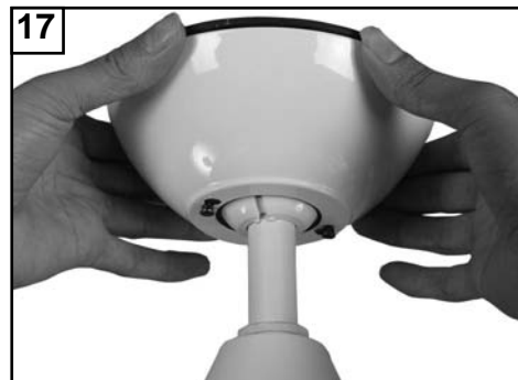
17 Raise the canopy up and align the two holes in the canopy with the two holes in the hanger bracket. Secure with two screws provided.
