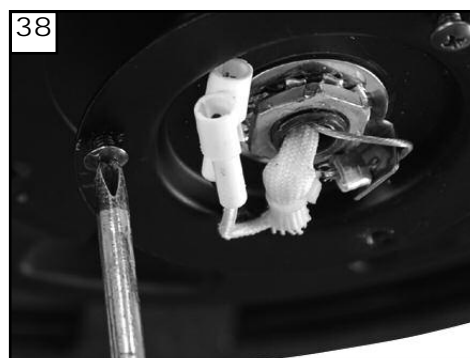
38 Loosen 2 screws and remove 1 screw. Save screw removed.
