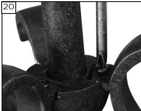
20 Install arch arms to arch hub using screws removed step 18.
