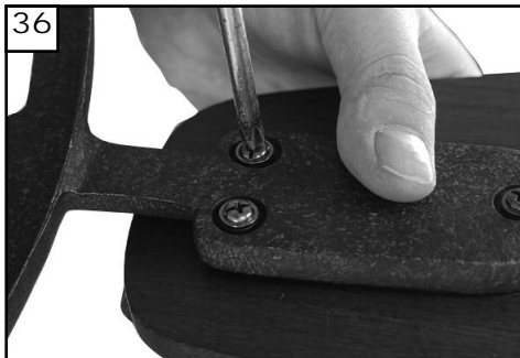
36 Check the motor for plastic shipping stabilizer tabs and remove if they are present. The screws, washers and motor pads are pre-installed to the blade holders. Attach blade assembly to motor and tighten screws securely.
