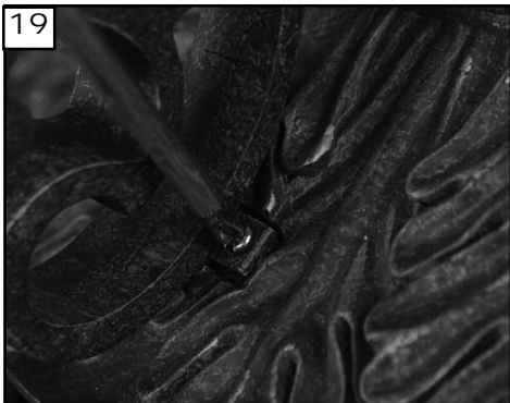
19 Install lower foot of arch arm with screws to fan upper housing.
