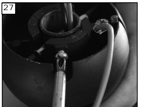
27 Tighten set screw to hold ball in place.
