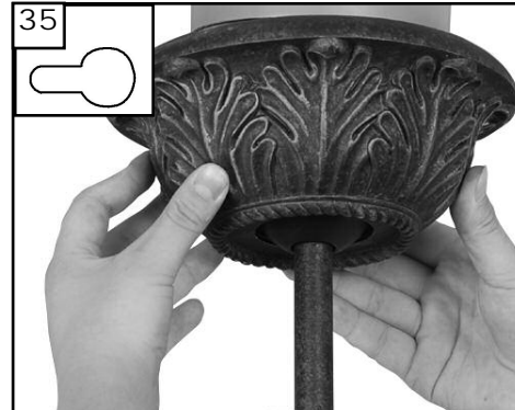
35 Lift canopy to ceiling aligning the key hole slots with the screws on the bottom of the mounting bracket. Rotate the canopy counter clockwise to lock in place. Tighten the screws to secure the canopy. See inset for keyhole shape
