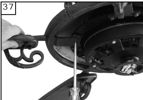
37 Check the motor for plastic shipping stabilizer tabs and remove if they are present. The screws, washers and motor pads are pre-installed to the blade holders. Attach blade assembly to motor and tighten screws securely.
