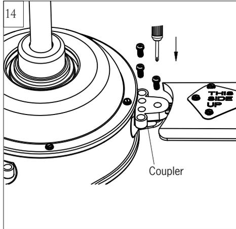
Install blade assembly. Align the holes on blade bracket with the screw holes on the coupler of flywheel, and install the blade assembly with set screws provided. Tighten screws securely. Repeat this process for remaining blade assemblies.
