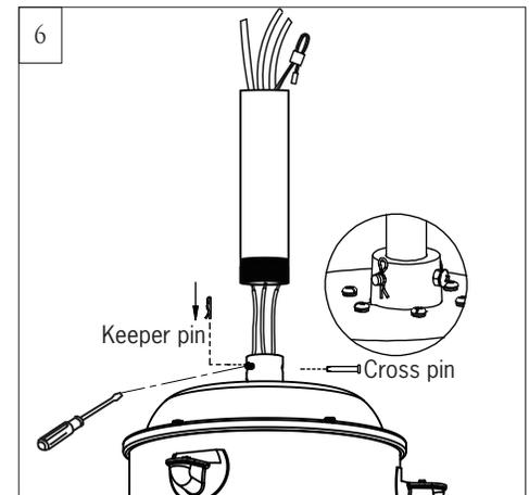
Thread lead wires and safety cable from motor assembly through downrod. Install downrod. Thread downrod into the yoke on top of fan until the holes on downrod are aligned with the holes on the yoke, and then install cross and keeper pins. Tighten the downrod set screw.
