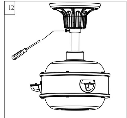
Lift canopy and fix it on downrod with the preinstalled set screw, tighten the screw securely. The canopy should adjust for any irregularity in the ceiling or outlet box.
