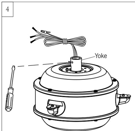
Partially loosen downrod set screw from yoke at top of the motor assembly.
