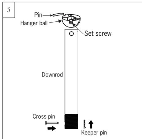
Remove hanger ball from downrod by loosening the set screw and removing the pin as shown in illustration. Keep parts. Remove preassembled keeper pin and cross pin from downrod. Keep parts
