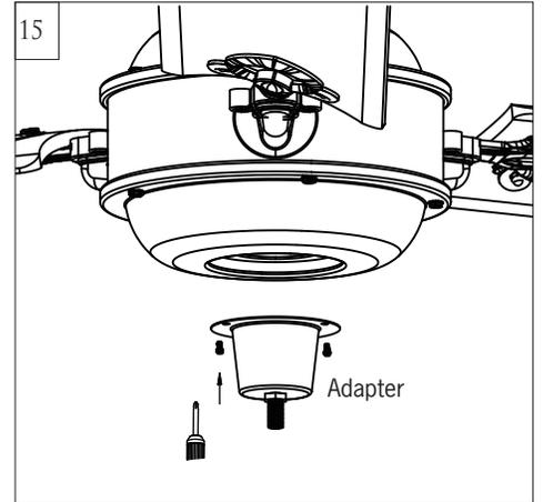
Install the adapter onto fan housing with set screws provided.
