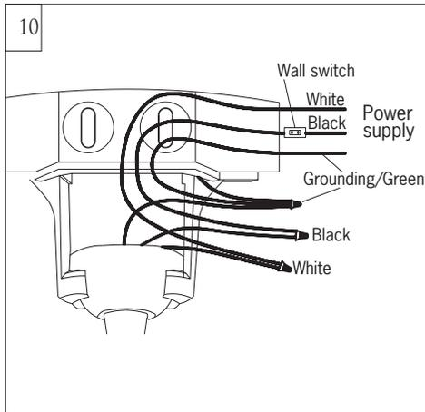
Make wiring connections as indicates above, using wire connectors provided. Connect Black wire from fan to Black (Live) wire from house. Connect White wire from Fan to White (Neutral) wire from house. Connect all green grounded wires to Grounded wire from House. Make sure that no filaments are outside of the wire connectors.
