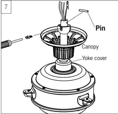
Place yoke cover and canopy over lead wires, safety cable and downrod, and then replace the hanger ball.
