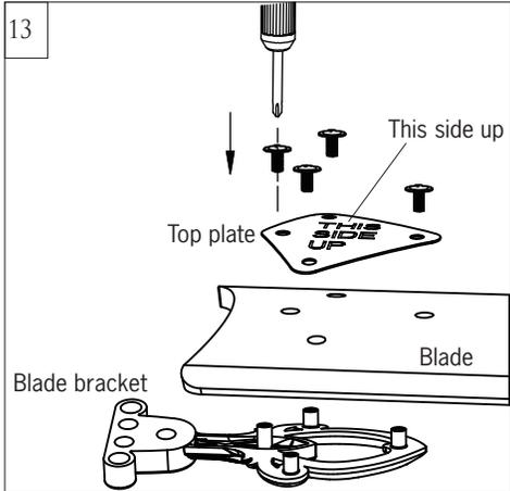
Install blade onto blade bracket with a top plate by 4 blade screws provided. Tighten screws securely. Repeat this process for remaining blades.
